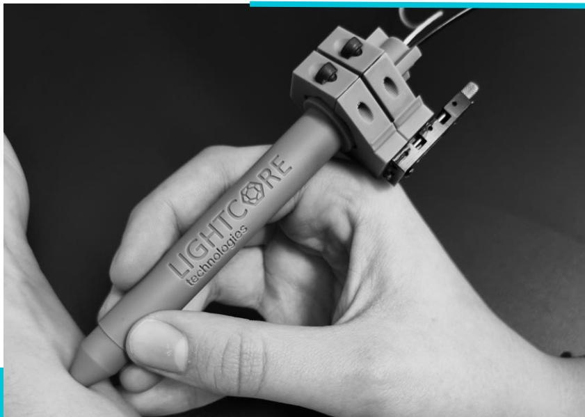
With our custom-made **hand-held** endoscope pen, and integrated **z-scan**, we are able to perform real-time in-vivo imaging
